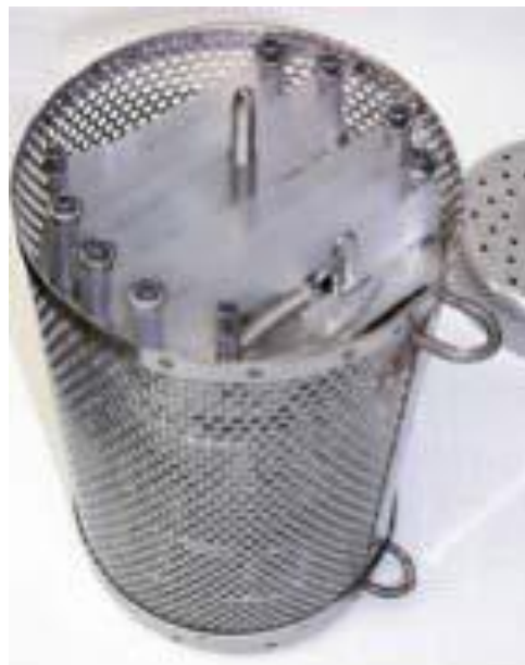
Figure 2-9 Semi-Permeable Membrane Device in Deployment Apparatus
