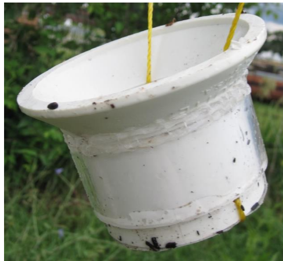
Figure 4-13 Bioretention Deployment Unit Influent Sampler Housing
